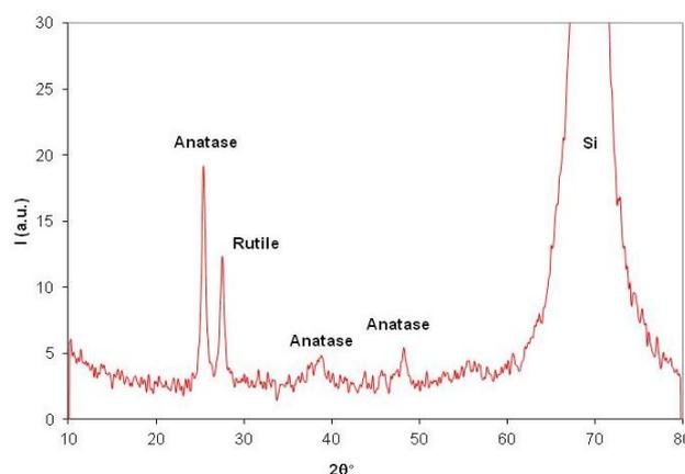
Fig. 1. XRD pattern of TiO<sub>2</sub> deposited on Silicon substrate (19 sccm of Ar and 1 sccm of O<sub>2</sub>).
