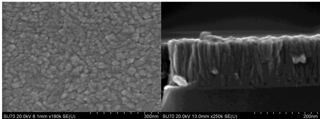
Fig. 2. Top (left) and cross-section (right) view SEM images of a TiO<sub>2</sub> coating.
