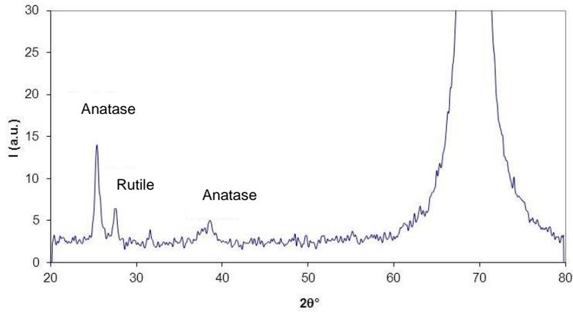
Fig. 4. XRD pattern of  $\text{TiO}_2$  deposited on Silicon substrate (19 sccm of Ar and 1 sccm of  $\text{O}_2$ ).
