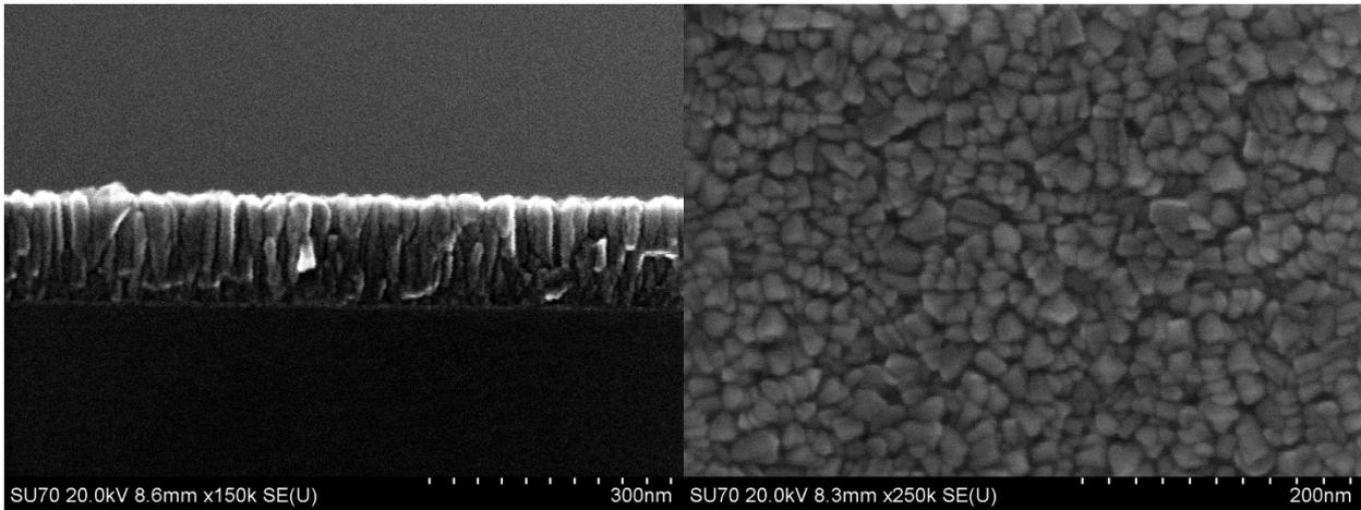
Fig. 5. Top (left) and cross-section (right) view SEM images of a  $\text{TiO}_2$  coating.
