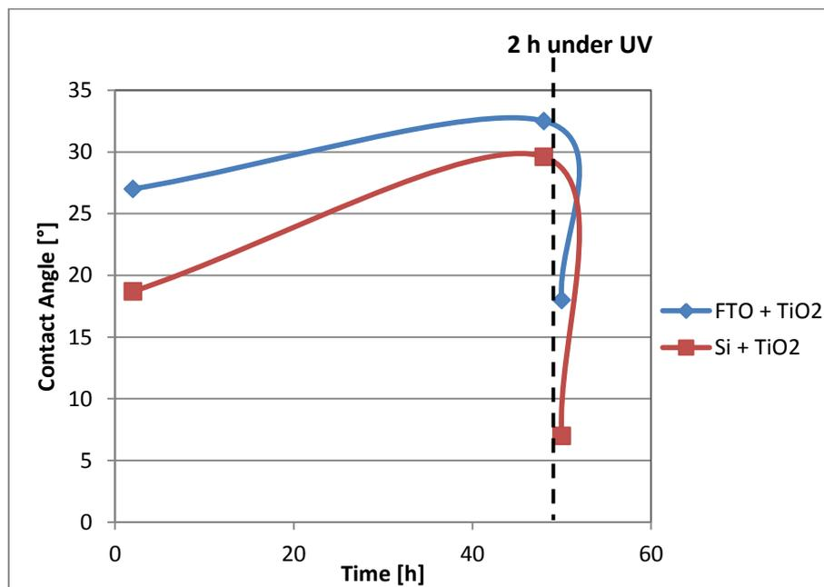
Fig. 3. Reversible trend of TiO<sub>2</sub> due to UV irradiation.
