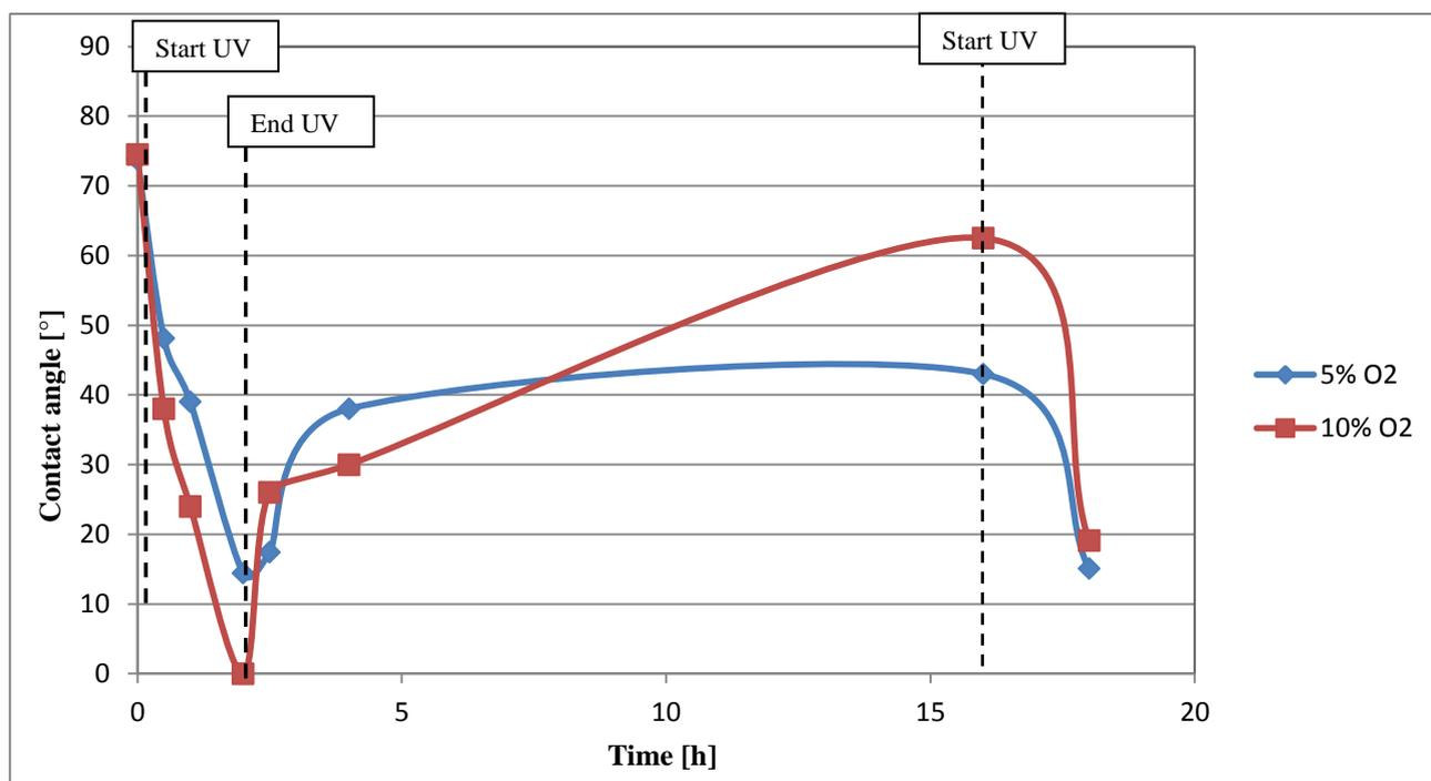
Fig. 6. Evolution of contact angle under UV illumination.
