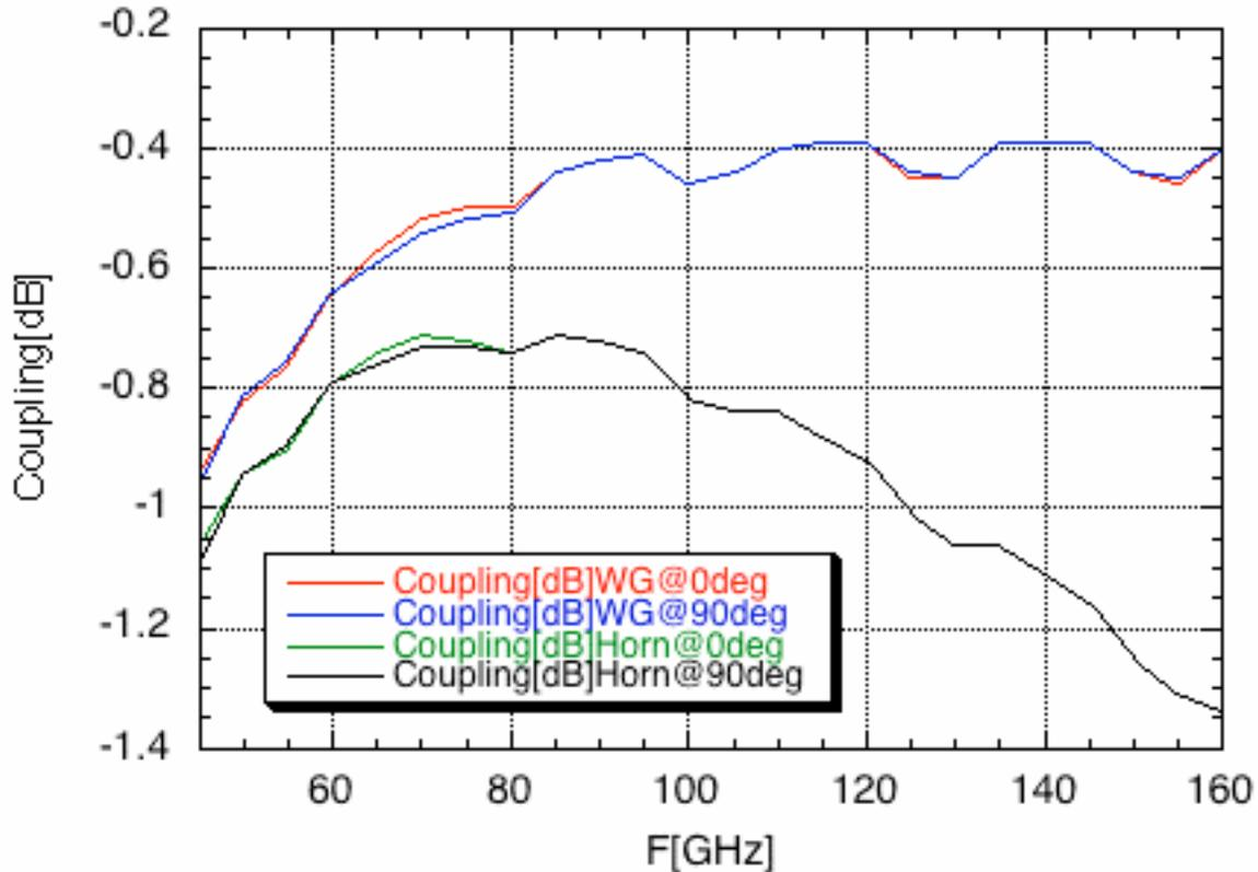
*Coupling between  $HE_{11}$  in corrugated waveguide and  $TE_{10}$  in rectangular waveguide (top curves) or 150mm horn (bottom ones) for the reference (TE) polarization and for a 90 degrees rotation into TM polarization. No significant difference is seen, as expected for the perpendicular reflection scheme.*
