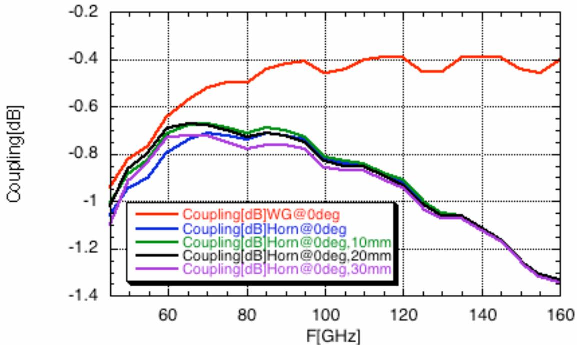
*Coupling between  $HE_{11}$  in corrugated waveguide and  $TE_{10}$  in rectangular waveguide (red trace, top) or 150mm horn (blue curve, bottom). The horn was displaced by 10 (green curve), 20 (black), 30 mm (purple) towards the mirror, to match the phasefront curvature of the Gaussian beam at least at one frequency. Best performance is for a displacement between 10 and 20mm.*
