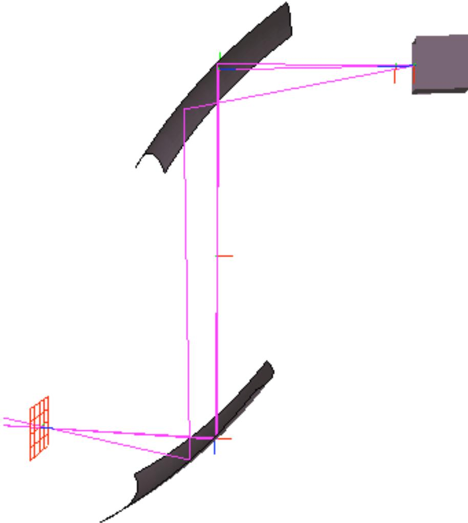
*Geometry of initial simulation. Top right the rectangular horn (simulated with a rectangular waveguide), reflection at two elliptical mirrors in confocal arrangement (center ray and one ray in either plane are shown) and the grid (bottom left) where the  $HE_{11}$  mode field is defined (computed externally).*
