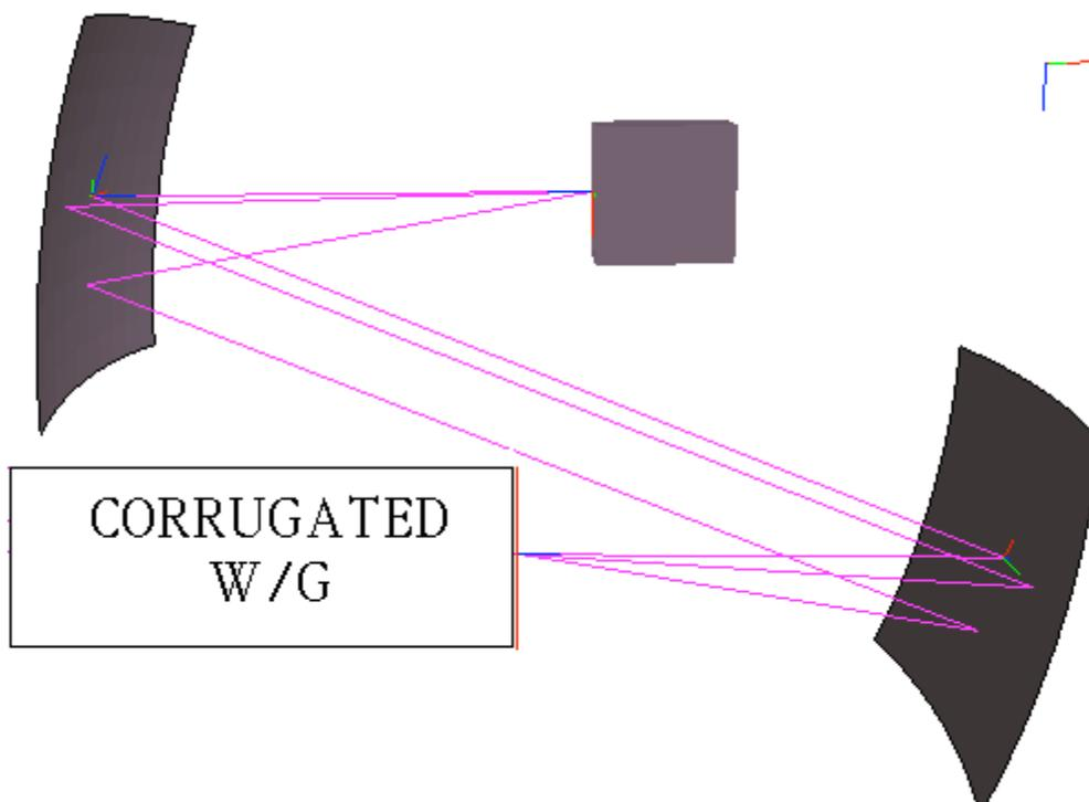
*Geometry of a transition with lower angle of incidence. The horn (rectangular waveguide) is top right, and three rays are shown per beam, the central one and one for each polarization plane.*
