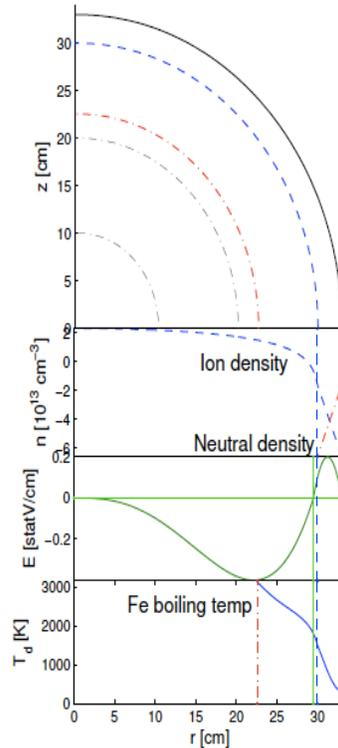
**FIGURE 1.** (top) Traces of relevant surfaces in the tokamak poloidal quadrant up to and across the LCMS (blue dashed line) (middle) ion and neutral density profiles; (bottom) radial electric field and electron temperature profiles, up to and within the SOL. .
