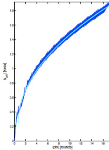
**FIGURE 3.** For the case of Fig.3 here the dependence is shown of the toroidal dust velocity (dark blue line) on the number N of toroidal loops, compared with the scaling  $N^{1/2}$  (light blue line).
