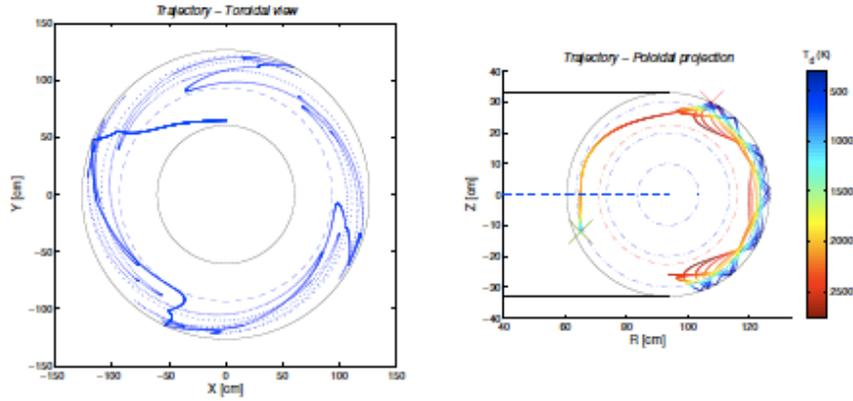
**FIGURE 2.** (left) projection in the equatorial plane of the FTU tokamak of the trajectory of a  $2\mu$  Fe dust particle; (right) projection in a meridian (poloidal) cross section
